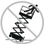
Do not drive the machine on or near uneven terrain, unstable surfaces or other hazardous conditions with the platform raised.
